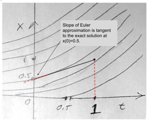
Line starts at (0, 0.5), slope is tangent at (0,0.5) and extends until endpoint lines up with t=1.
