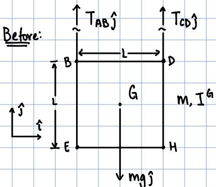
By symmetry and inspection  $\Rightarrow T_{AB} = T_{CD} = \frac{mg}{2} \star$
